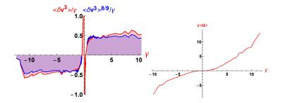
Scalings / circulation (left red):  $u^3 \sim \Gamma \gamma$ Scalings / energy: Sedov-Taylor (left blue)  $u^8 \sim E \gamma^3$ ; Scaling Kolmogorov (right)  $u\gamma \sim \epsilon$  on the right Notice: Taylor frozen turbulence does not apply because the large velocity fluctuations are of the same order as mean velocity.
